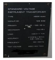
Fig. 1. Nameplate of reference VT
